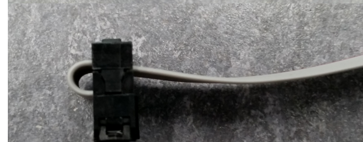
4. Fold cable around, clip in strain relief
