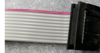
1. Place ribbon cable and press together
