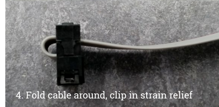
3. Fold cable around, clip in strain relief
