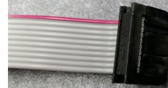
1. Place ribbon cable and press together
