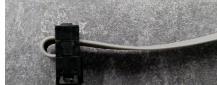
4. Fold cable around, clip in strain relief
